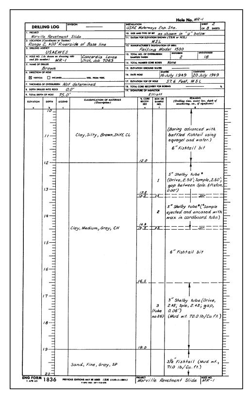
Figure 13-2. ENG Form 1836 for maintaining a record of drilling and undisturbed sampling operations
